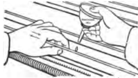
FIG. 77. — OILING WAYS OF A MACHINE.
